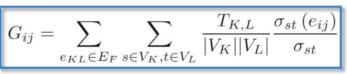
We assume that the transport of natural gas occurs along the shortest path in geographical We generalized space. centrality by weighting betweenness estimated gas flows per pipeline.
