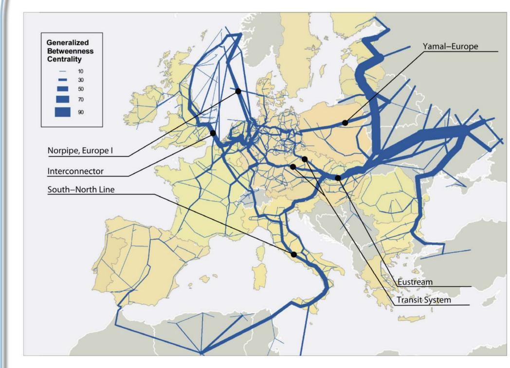
Link thickness proportional the to generalized betweenness centrality; We labeled several major EU pipeline connections;
