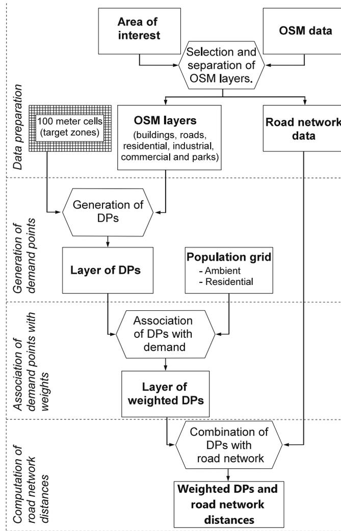
Figure 2. Work-flow of input data processing for the service system design problem from OSM data and population grids.
