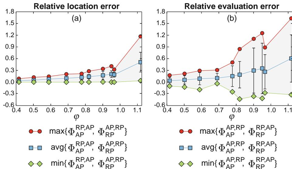
Figure 6. The maximal, minimal and average relative location and evaluation errors as a function of the parameter  $\varphi$ . Maximum, minimum and average values are for a given  $\varphi$  (i.e. for a given district) calculated from the results of all experiments, where  $p = 1, \dots, 40$ . Error bars are reflecting the standard deviation around the average.
